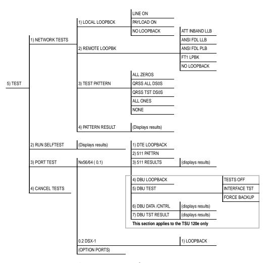
Figure 7-1. Complete Test Menu Tree
